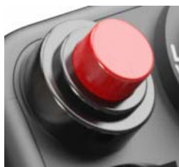
Temporary push button
